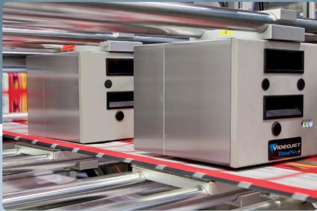
The Videojet DataFlex Plus Thermal Transfer Overprinter (TTO) delivers high resolution images on flexible packaging, while minimizing downtime and costs associated with ribbon breaks and production changeovers. For marking variable information such as date, time, batch code, ingredients, logos and marketing information onto flexible film packaging, labels or glossy cards, this system provides the ultimate in productivity and efficiency.
